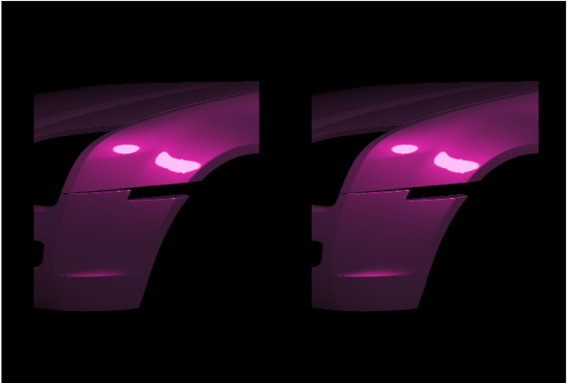
Figure 4.6: Bumper and fender misaligned by 8 degrees. Identical metallic paints cause a color mismatch (left) while painting the bumper a different color, determined using the inverse trompe l'oeil technique, eliminates the problem (right).
