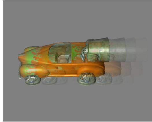
Figure 1: Ghosting or temporal aliasing effect when the motion blur of a fast moving object is generated using accumulation buffer but large time interval between multiple renderings.
